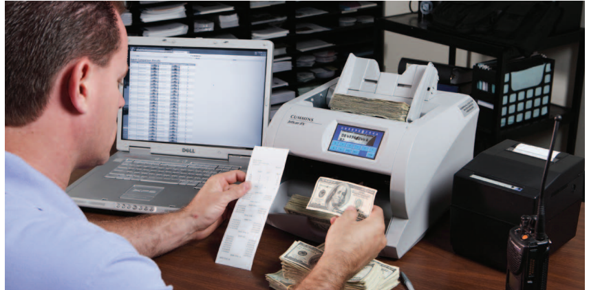
The JetScan iFX generates a print-out detailing the count and serial number.
